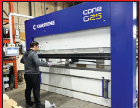
G25 - 8 FT x 89 TON 6 Axis, 2D Graphics, Laser Guards, CNC Ram Crowning, Hyd. Tool Holders
