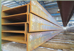
Wide Flange Beams
